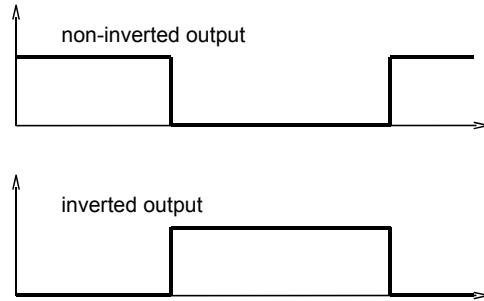
A Power-On delay function (ordered as a separate option) makes it possible to maintain the switching output in the normal state for a defined period after application of the supply voltage.
