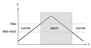
A switchover delay time  $(t_{\mbox{\scriptsize DS}})$  can be applied to the switchover to the alarm state. Equally, one switch-back delay time ( $t_{\text{DR}}$ ) of several can be applied to switching back to the normal state.
