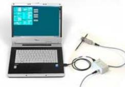
If required, all parameters can be set at any time on all intelligent sensors, using the ECI-1 device configurator.
